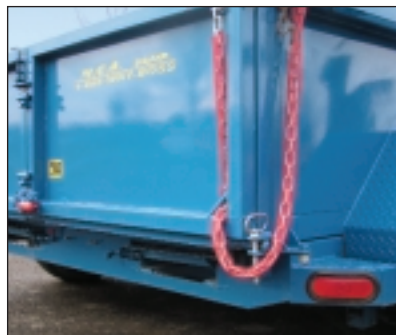
Slide-out ramps store easily on lower frame. Taillights are positioned on the sides to prevent damage when dumping.
